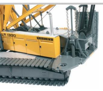
The frame of the ballast carrier is highly detailed and functional, with walkways fitted along the top of the extending arm, complete with integrated access ladder and safety railings, not to mention the flexible hydraulic hoses. The four axles have simulated, nonfunctional suspension detailing with four wheels fitted to each axle, complete with rubber tyres that have a grooved tread pattern. Two large stabilisers are also integrated into the tray, and are extendable simply by pulling them out.
