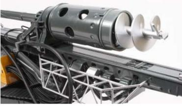
tasks including Kelly drilling, continuous flight auger drilling, double rotary, soil mixing and drilling with partial or full displacement tools. Powered by a 469hp D846A7 diesel engine with a working weight of 96 tonnes, the machine is custom-designed for most drilling applications, and the 1/50 model from NZG has captured the features of the full sized machine very well.
