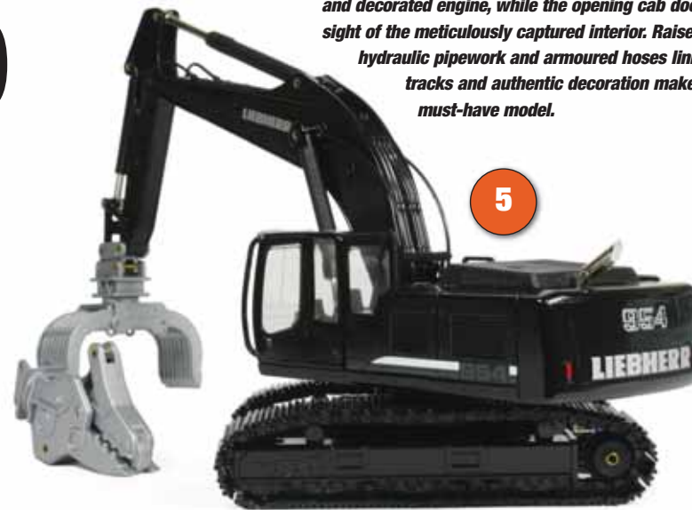
5: The Liebherr R954C has also been produced in a special black colour scheme with silver printing. In addition, there is a new quick coupler attachment fitted to the stick to allow two different demolition attachments to be deployed – a concrete pulveriser and a sorting grapple – which both feature 360-degree rotation and opening jaws.
