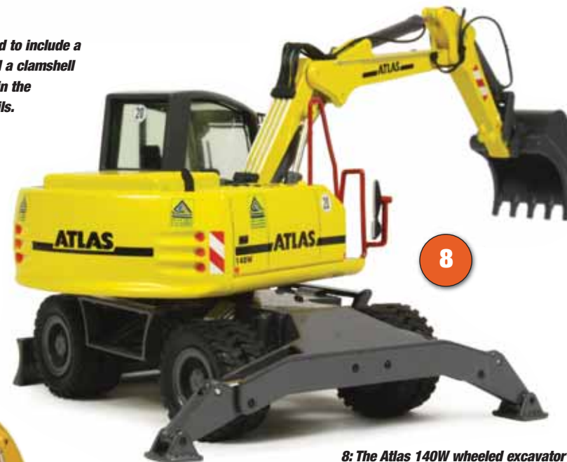
8: The Atlas 140W wheeled excavator from NZG has appeared in the yellow colours of German firm Bleck & Sohne with an excellent paint finish and crisply applied graphics throughout adding to the authentic look. The undercarriage features working blade and outriggers with a steering axle while the digging equipment consists of a two-section hydraulically adjustable boom and general-purpose bucket.
