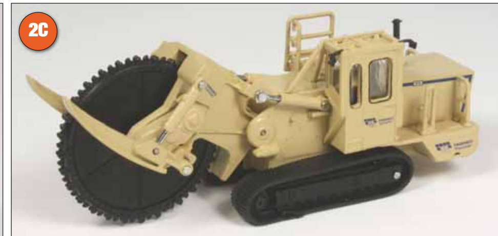
2A, 2B and 2C: The 975 rock saw has an interesting appearance and is ideal for cutting narrow trenches in hard rock and concrete. It is the only model in the set that has functional parts, allowing the cutter wheel to be lowered while the side support arms can also be adjusted. The wheel has good detailing of the cutting teeth and rotates, while the body has good structural support details, complete with safety railings and a large textured engine grille.
