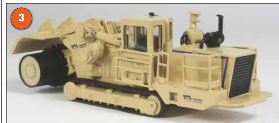
1A, 1B and 1C: The most detailed model in terms of appearance is the 885 chainsaw trencher, which has a non-functioning flexible cutter chain topped with raised teeth along with a pivoting upper guard. The main body houses a spoil removal conveyor that allows material to be deposited to either side of the chassis while the optional rear discharge conveyor has also been included on the model, demonstrating the ability to load trucks at the front of the trencher when working in confined spaces. The high position of the cab offers a good view of the worksite and the level of detail, from the painted window seals, engine grille and fully modelled hydraulic drive for the chain highlight what is possible to add to such a small model.
