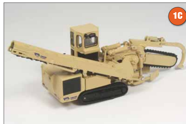
1A, 1B and 1C: The most detailed model in terms of appearance is the 885 chainsaw trencher, which has a non-functioning flexible cutter chain topped with raised teeth along with a pivoting upper guard. The main body houses a spoil removal conveyor that allows material to be deposited to either side of the chassis while the optional rear discharge conveyor has also been included on the model, demonstrating the ability to load trucks at the front of the trencher when working in confined spaces. The high position of the cab offers a good view of the worksite and the level of detail, from the painted window seals, engine grille and fully modelled hydraulic drive for the chain highlight what is possible to add to such a small model.
