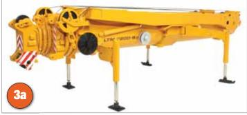
3 and 3a: Just like the full-size model, the fully functional telescopic boom assembly can be separated from the carrier on integrated support legs to demonstrate the ease of transport. The individual counterweight segments lock into place to keep the model balanced, as the weight of the jib with the extension on this model is not insignificant.
