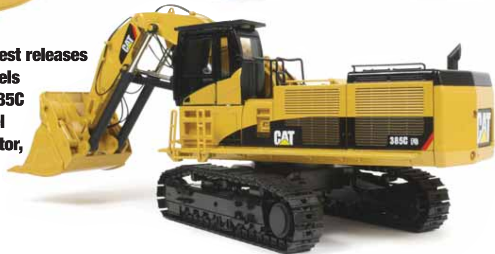
1: The 385C face shovel accurately captures all the details of the full-size machine very well, from the functioning shovel with hydraulic operated actuation, replicated tooth and wear plating, and flexible hoses to the protective covers over the stick and boom cylinders. The range of movement of the digging equipment is authentic, with narrow gauge track pads typical for quarrying applications and a high-rise cab offering a good all-round view.
