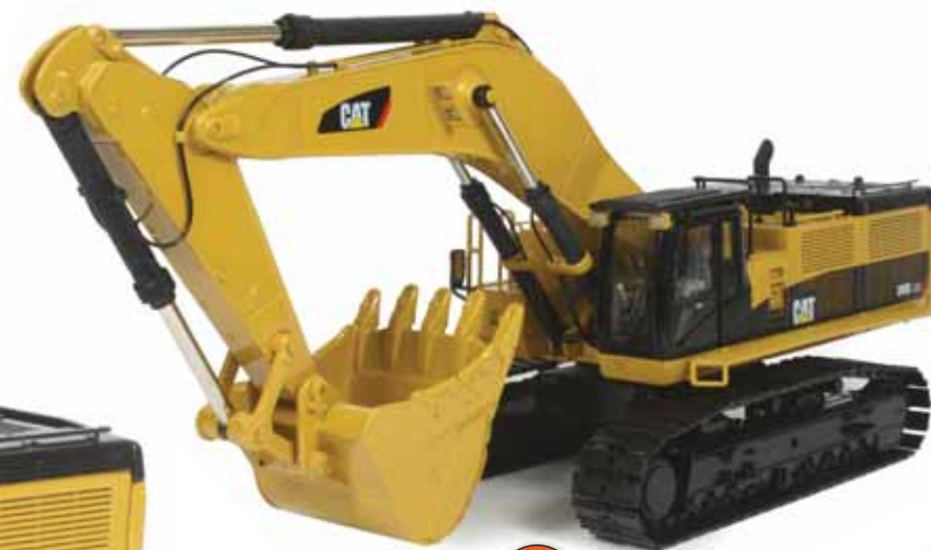
3: The 390D features a 7.25m boom and, for mass excavation work, is fitted with a large bucket with excellent cutting edge detailing and caps covering the connecting pins. The track pads installed on the undercarriage are wider than those fitted to the shovel version, and raised fixing bolt heads are visible on each pad.
