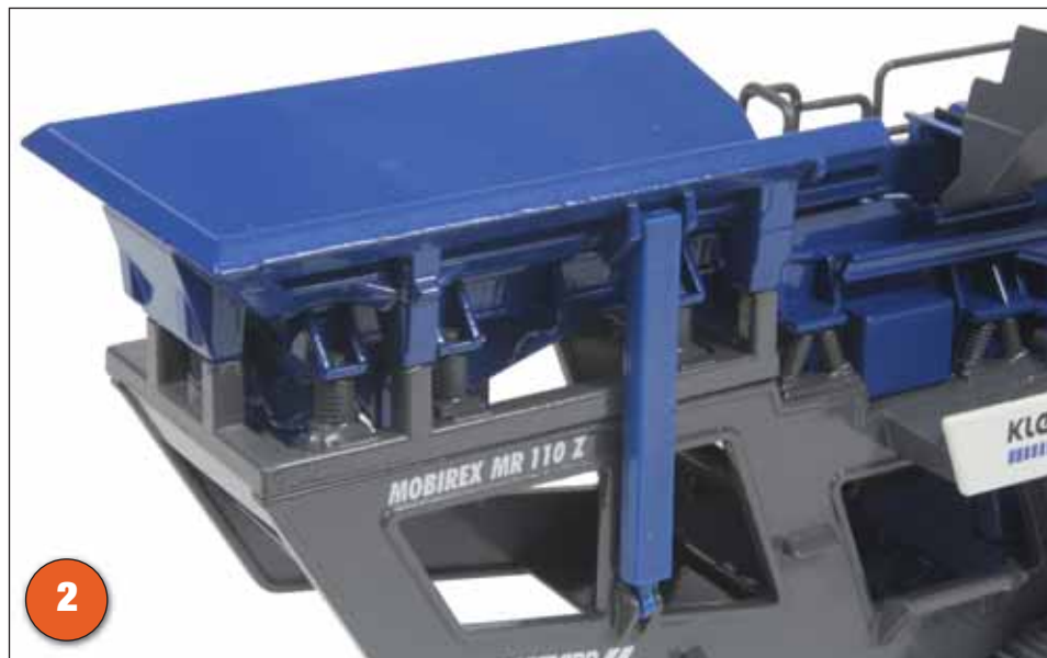
2: The hopper and vibrating feeder both have spring isolating mounts visible and motor housings located on the underside of the main frame. A natural fines conveyor is supplied and this can be fitted to either side of the chassis while a return conveyor has been fitted to the frame, which can be deployed to grade the material or return oversized material back into the crusher.
