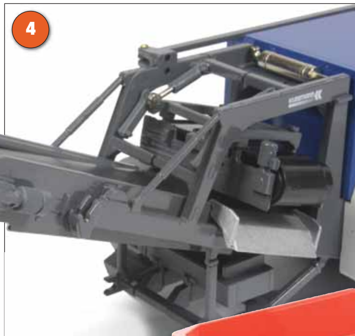
5 and 5a: The impact crusher housing has all the structural detailing presented, with an adjustable opening to allow larger material the flow into the throat. Flexible rubber strips have been fixed to the lip of the opening, simulating the covers on the full-size unit to prevent material from being thrown back.
