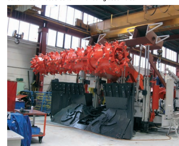
Sandvik continuous bolter miner being assembled
