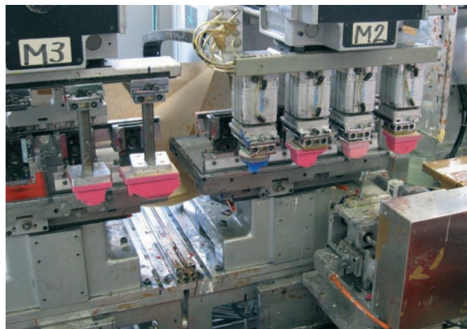
16-colour printing machine at work printing the cab
