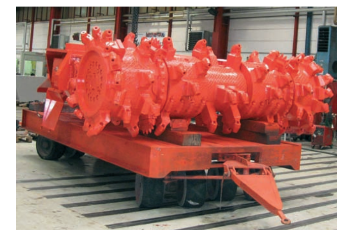
Sandvik borer miner cutter assembly
