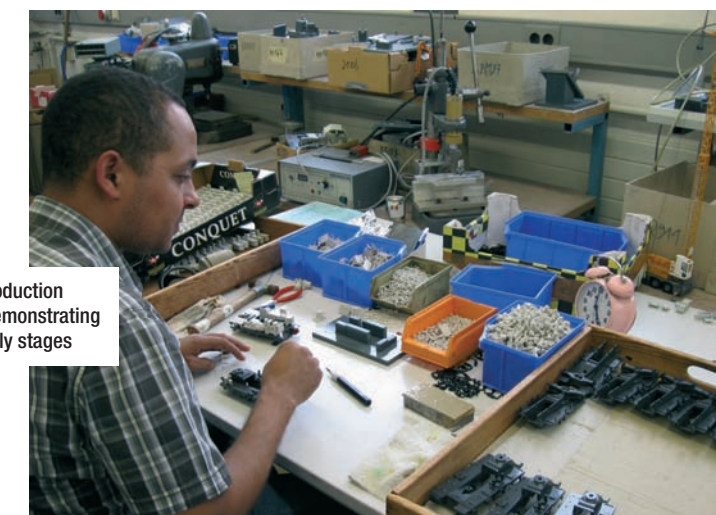
Cab and upper structure sub-assembly
