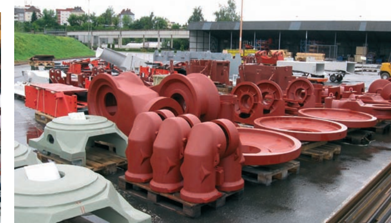
Outside storage area for the manufactured castings before final machining
