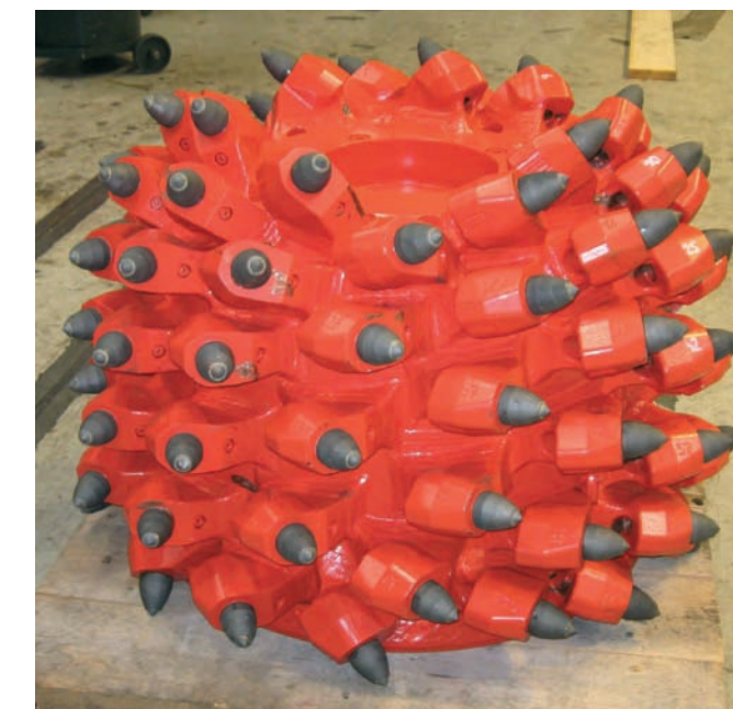
Sandvik roadheader cutter assembly
