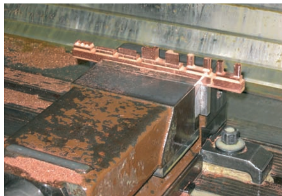
Copper master being machined
