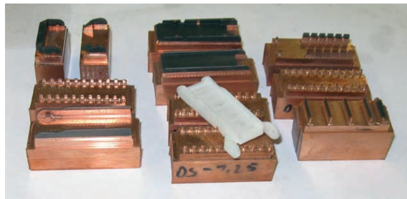
Set of copper masters which produce the base section of the conveyor
