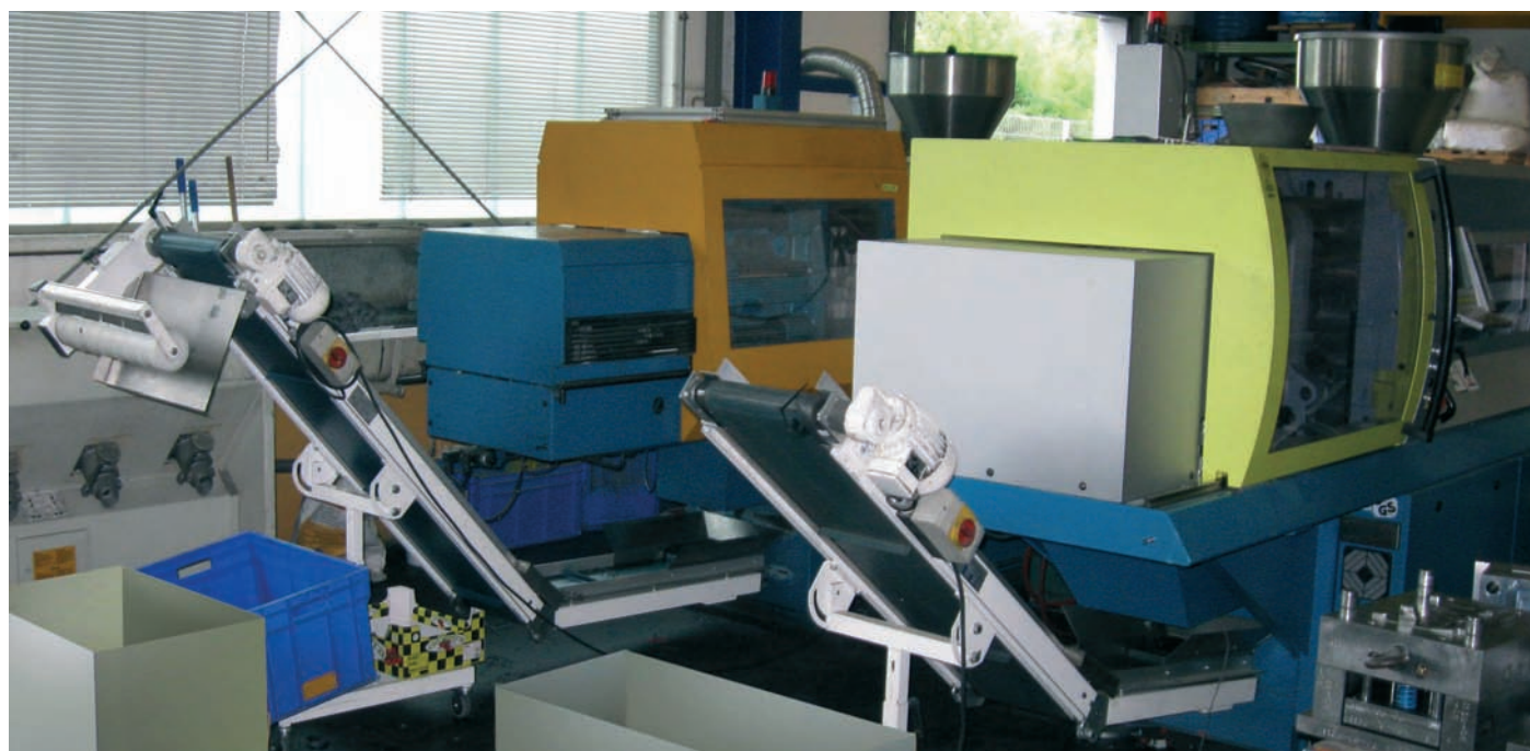
Two of the plastic injection moulding machines busy producing the MT720 track pads and white plastic components
