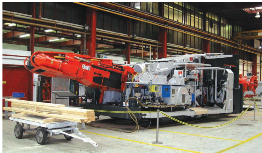
Sandvik continuous bolter miner final assembly
