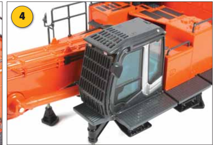
4: The cab has very good, crisp detailing of the roof and front debris protection screens, which are fitted to the frame and house integrated work lights, while the printed window seals and fully replicated interior all add to the realism.
