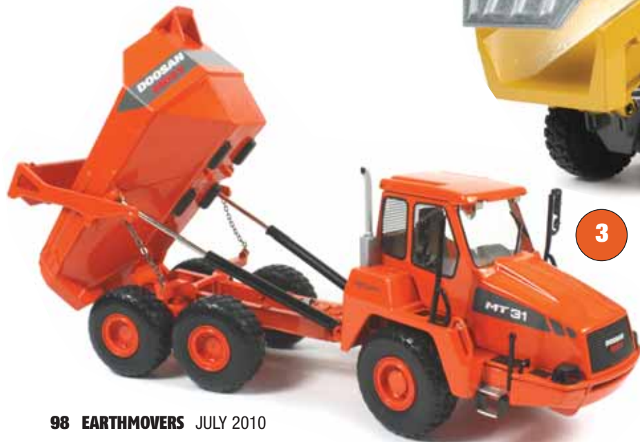
3: Doosan has commissioned a limited edition version of its Moxey MT31 articulated dump truck from NZG, which features a new orange paint scheme with updated and revised decals. The chassis features working suspension and steering with a replicated cab interior, safety rails, rear view mirrors, tipping dump body and chain-operated tailgate.
