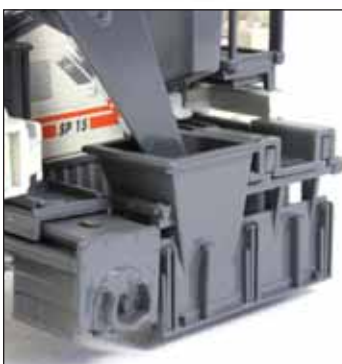
1: The American specification SP15 slipform paver is the smallest in the range of Wirtgen offset concrete pavers, capable of forming various continuous concrete profiles for rapid construction of kerbs, gutters and waterways. The 1:50th-scale model from NZG has accurately captured the functionality of the full-size machine. The model is available in two versions – with a conveyor belt or an auger feed. Both feed concrete into the hopper of the mould, which can be positioned on either side of the chassis and has the ability to extend for more flexibility. The model is fitted with a trimmer unit, complete with rotating cutter drum and auger spoil transfer, which extends from the chassis and lowers to provide an even sub-grade level.
