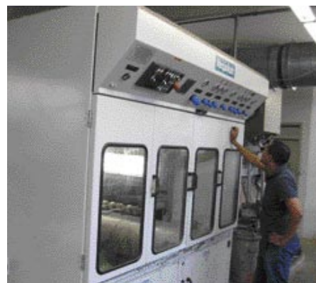
A worker monitors the pressures, making adjustments for a perfect paint finish.
