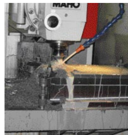
Machining of the main structural components of the mould is the first step.
