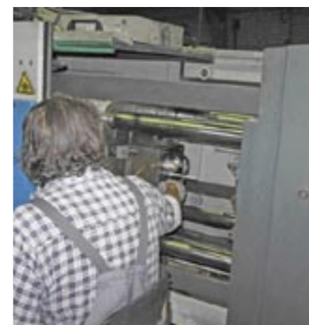
A worker carefully removes the fragile parts from the casting machine to prevent damage while the parts cool.
