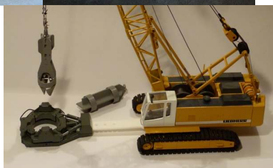
Extension for casing oscillator (kit) between casing oscillator and HS843HD duty cycle crawler crane
