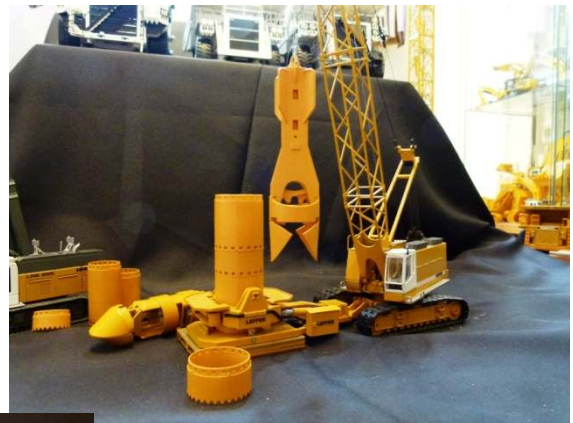
Hammer grab ø2000 and casings in combination with the casing oscillator by HiMoBo and the HS885HD by Conrad
